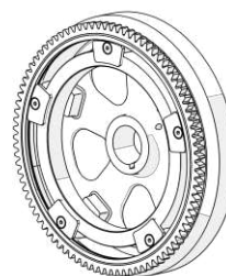
Fig. 2: Lower flywheel with rotor (part no. 304711)
